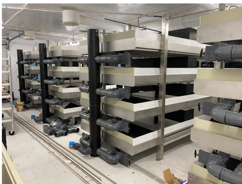
Figure 6.1.a: The tipper system (based on the abalone tipper systems) installed at the Stavanger Facility.
