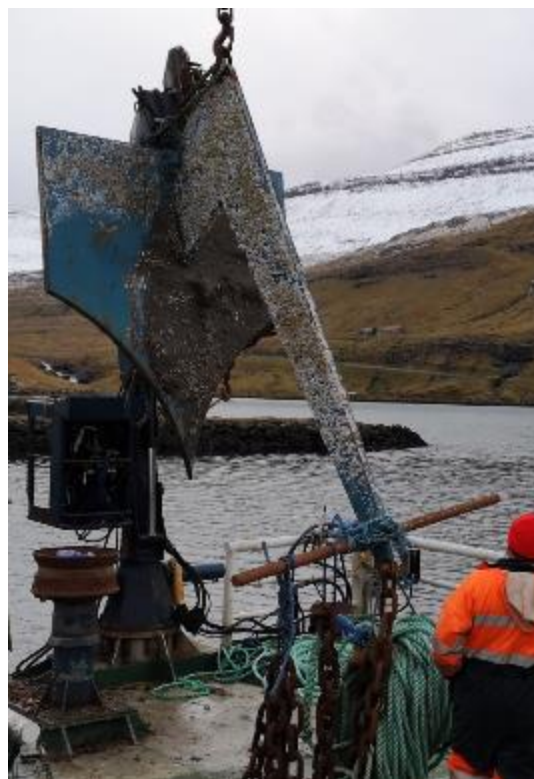
Figure 2.2.d: Handling of second-hand 1.5 tonnes steel anchors on the vessel Tongul in Funningsfjørður.
