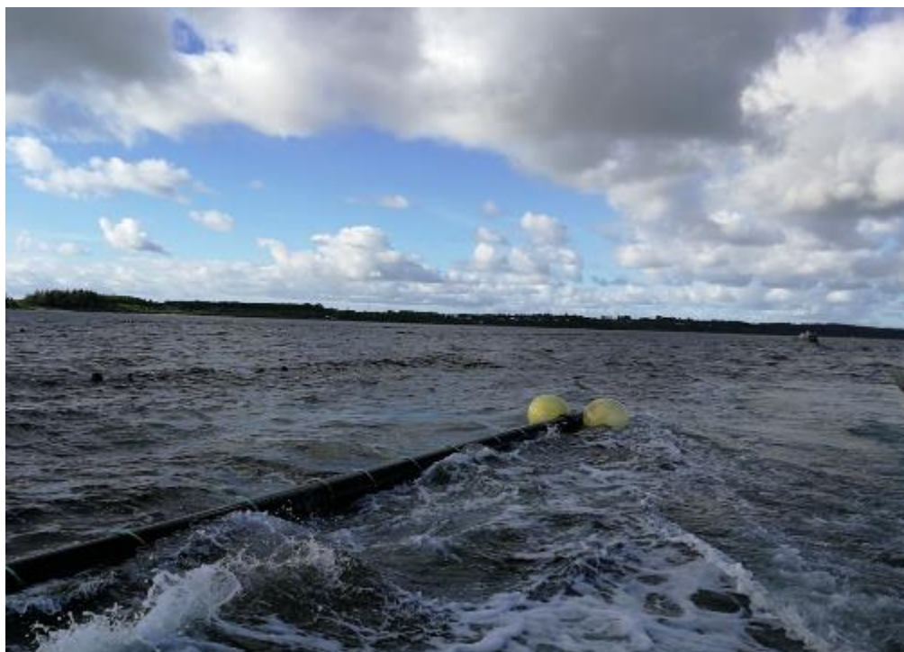
Figure 9.3.a: Submersible tube deployed at the DTU mussel farm. The tube is kept elevated at outlet side
