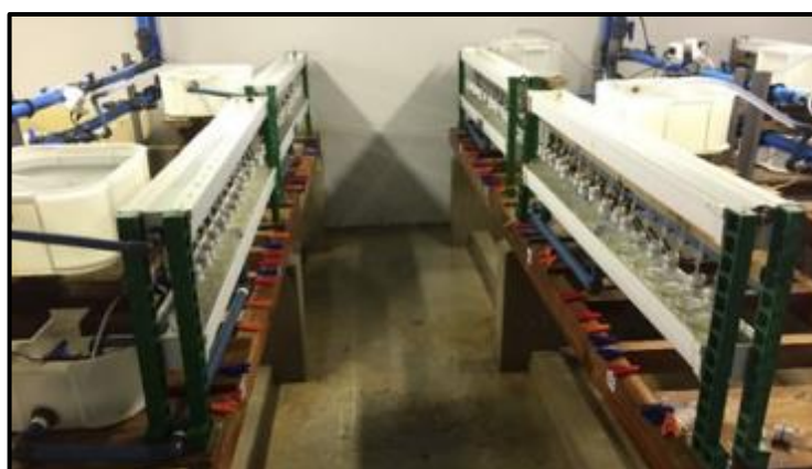
Figure 3.1.r: Four of the five experimental systems designed and built for the trials carried out for this task. This figure depicts the system prior to larval inoculation, when plates were being treated – as indicated by the multicoloured pegs which were used to mark plates and their respective treatments after randomisation had been carried out.
