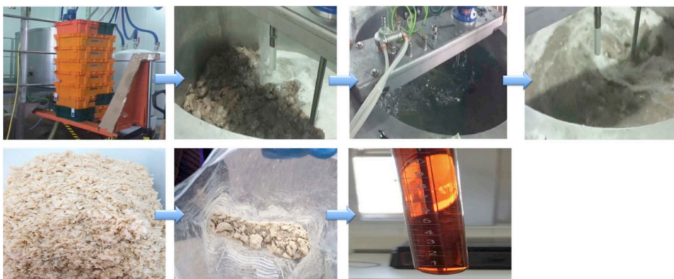
Figure 12.3.f: Steps of enzymatic hydrolysis of fish discards to produce FPH and oil in iDVP3.
