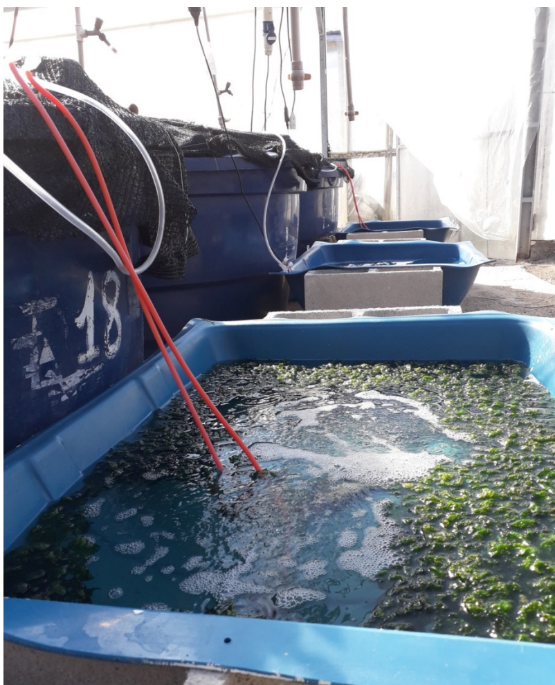
Figure 5.2.b: Experimental design used for the evaluation of two stocking densities of Ulva ohnoi (2 and 4gL -1 ) using effluent from a biofloc shrimp rearing unit.
