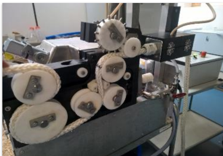
Figure 2.3.c: A mechanical seeding device developed by IHC and Hortimare.
