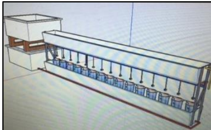
Figure 3.1.q: Concept design of the systems to be built for the settlement induction trials.
