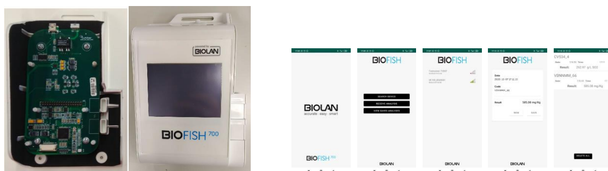
Figure 5: Detail of the device, the PCB and the developed App
