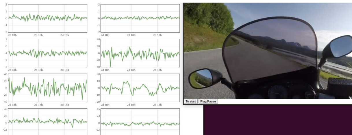
Figure 9: Screenshot from data capture. X=time, Y= individual movement along a given axis.
